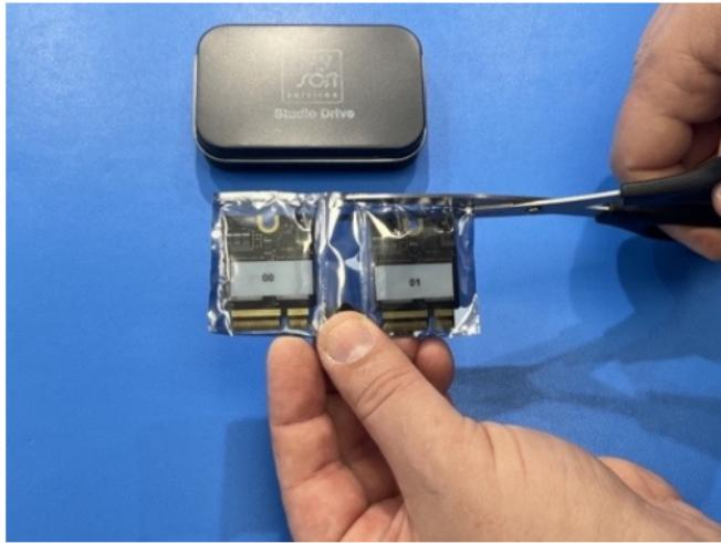
The 2TB kit is only 1 card which goes in slot 00, while the 4TB, 8TB and 16TB kits consist of 2 cards going in slot 00 and 01, with a new screw for the 2 card :
