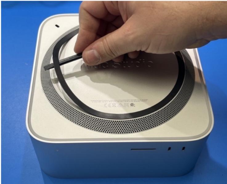
Remove the 4 screws from the bottom cover using the T10 bit and screwdriver :
