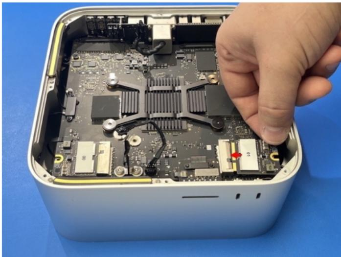
Replace the SSD screws with T8 bit and screwdriver :
