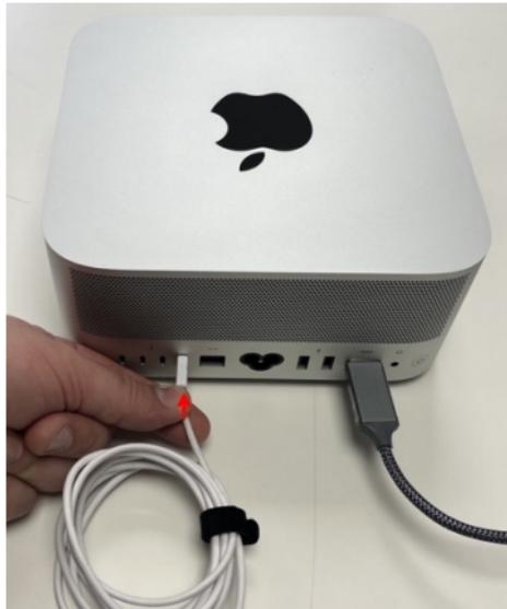
Now for the tricky part : place your Mac Studio in DFU mode. Do this by first pressing and holding the power button, and then and while still pressing the power button, plug the AC mains cable :
