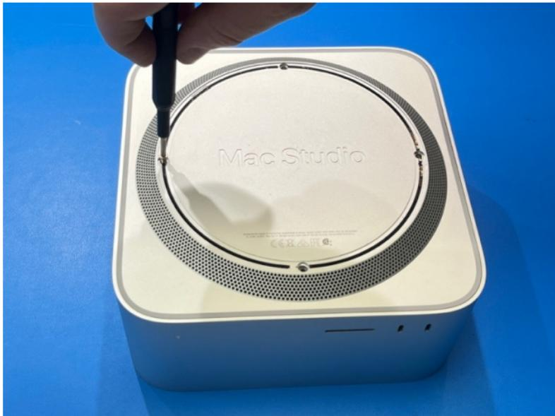
Then put the screw cover back on, making sure that the smoother surface faces upwards :
