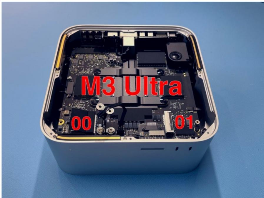
Place the new Studio Drive "00" module by gently sliding it sideways into slot 00 :
