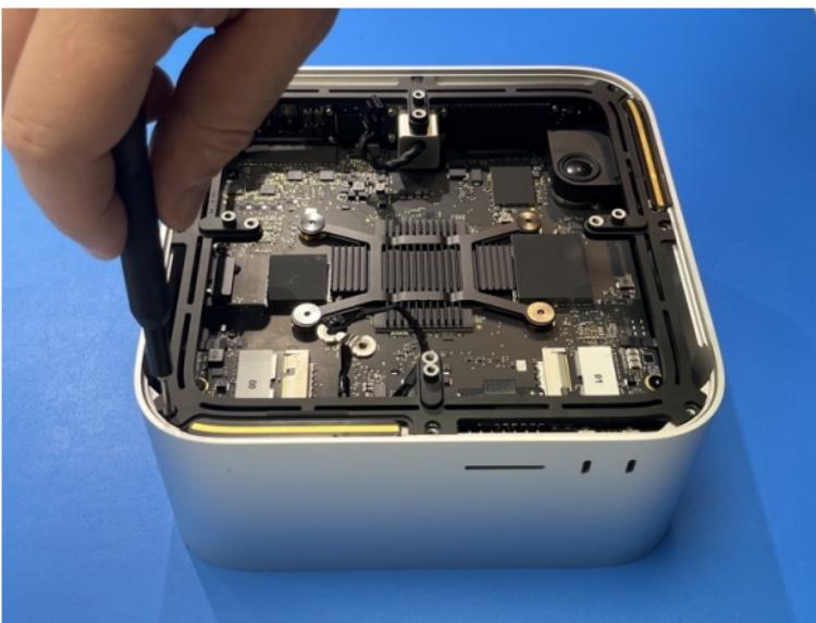
Finish by the short screw on top of the AC socket :
