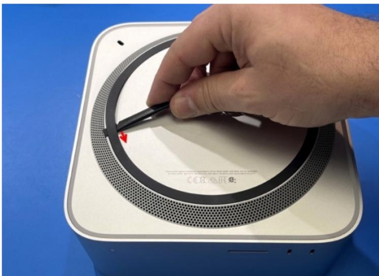
You can now lift the circular screw cover. On the M3 Ultra Mac studio, the screw cover adhesive can be reused so please don't damage it.
