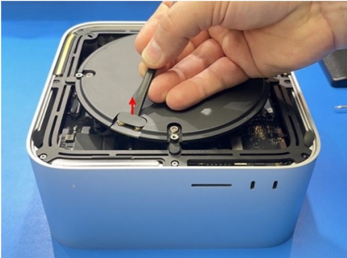
Then remove the 2x bus bar screws using the T10 bit and screwdriver :
