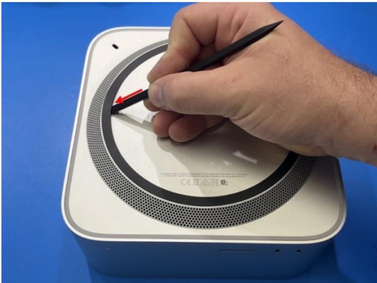
Then move around the nylon tool to unstuck the circular screw cover :
