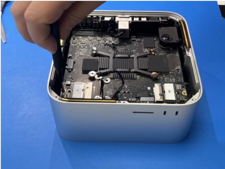
for 4TB, 8TB and 16TB kits, use the supplied new screw for the second module :
