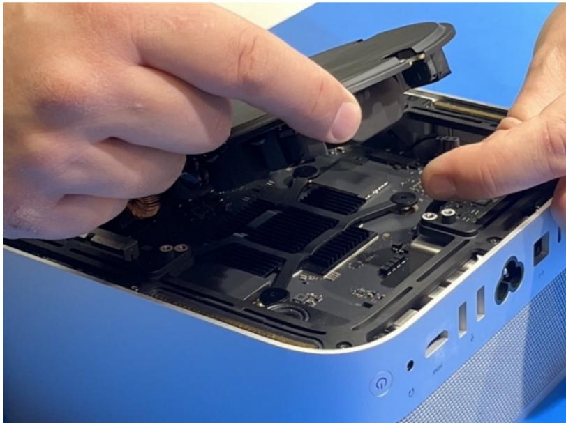
Fully lift up the power supply unit, pinch the data signal cable clip and pull it out of its connector, **please be carefull to not rip the data signal connector !**
