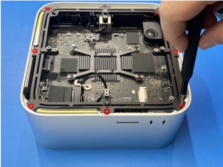
Remove separately the shorter 8<sup>th</sup> screw which is above the mains socket :
