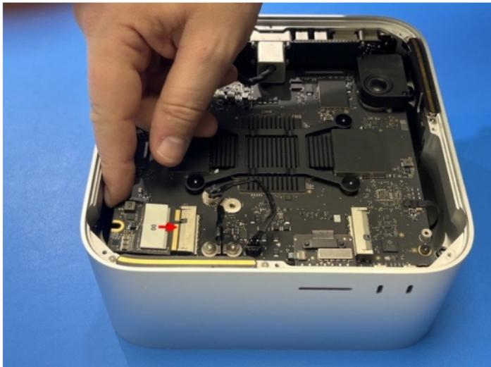
for 4TB, 8TB and 16TB kits, install the 2nd module in slot 01 :
